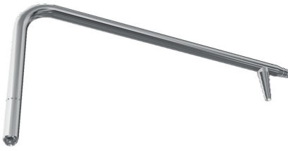
Fig. 9.3. Prandtl's pitot tube
