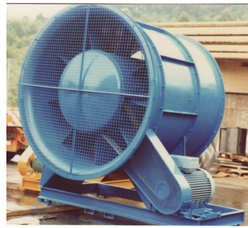
Fig. 5.20. Belt-driven axial fan on the base frame
