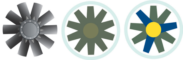
Fig. 5.12. Axial impeller, diagram showing different arrangements of blades on hub
