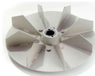
Fig. 5.25. Impeller with radially ending blades :
