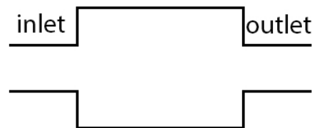
Fig. 4.7. Example of reactive silencer
