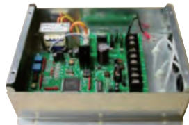
Relay Interface BMS-IFLSV4E For TCS-NET (Max. 64 FCU/Unit)
